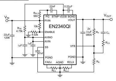
**Figure 5. Single Input Supply Schematic**
