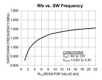
Figure 9. Typical R<sub>FS</sub> vs. Switching Frequency
