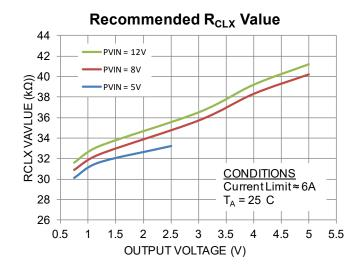
Figure 10. Typical RCLX vs. Output Voltage
