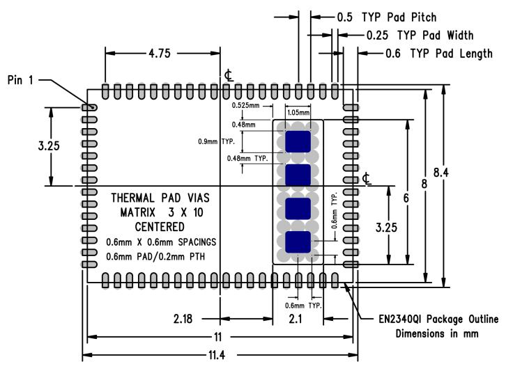
Figure 16. EN2340QI PCB Footprint (Top View)
