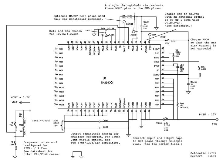
Figure 13. Engineering Schematic with Engineering Notes
