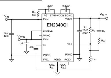
Figure 7. Dual Input Supply Schematic
