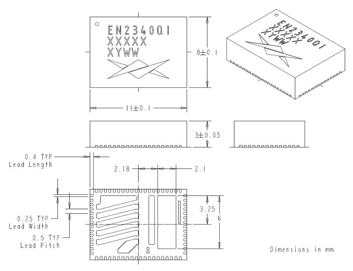
Figure 17. EN2340QI Package Dimensions (Bottom View)
