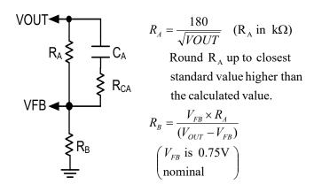
Figure 11. External Feedback Compensation. See Table 6 for details
