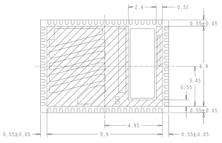
Figure 15. Lead-Frame exposed metal (Bottom View)
