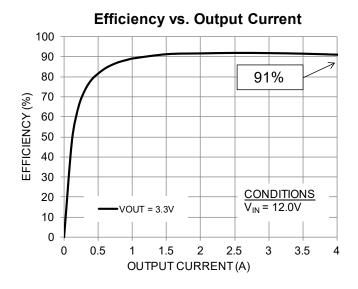
Figure 12. Efficiency vs. Output Current
