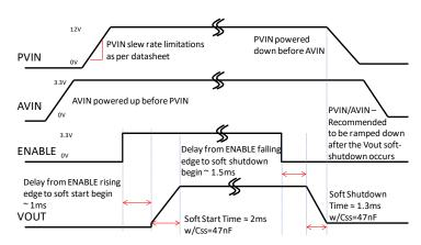
Figure 8. Dual Supply Startup/Shutdown Sequencing
