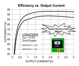
Figure 2. Highest Efficiency in Smallest Solution Size
