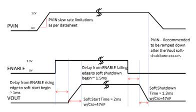
Figure 6. Single Supply Startup/Shutdown Sequence
