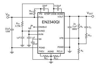
Figure 1. Simplified Application Circuit (Footprint Optimized)
