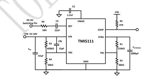
Figure 1. Basic Application Circuit
