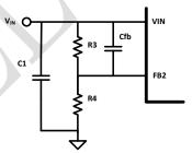
Figure 3. Feedback Divider Circuit for Release Voltage
