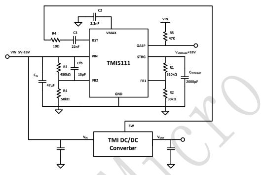
Figure 4. TMI5111 Typical Application Circuit
