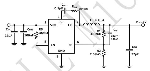
Figure 4. 12V<sub>IN</sub>, 5V/2A Output
