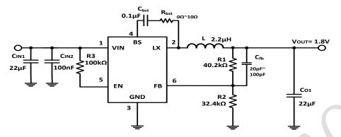
Figure 6. 12V<sub>IN</sub>, 1.8V/2A Output
