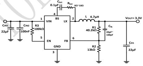
Figure 5. 12V<sub>IN</sub>, 3.3V/2A Output
