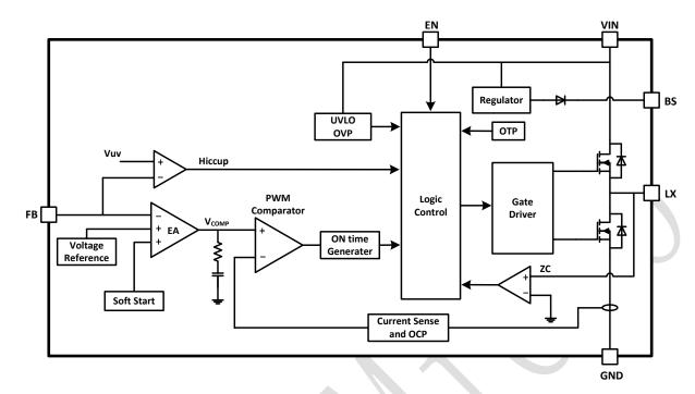
Figure 1. TMI3257 Block Diagram
