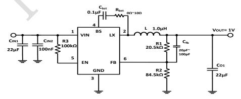
Figure 9. 12V<sub>IN</sub>, 1V/2A Output
