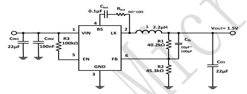
Figure 7. 12V<sub>IN</sub>, 1.5V/2A Output
