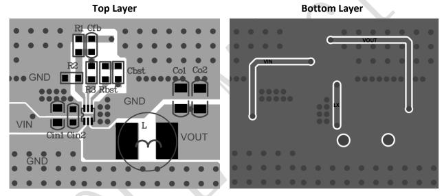
Figure 3. Sample of PCB Layout
