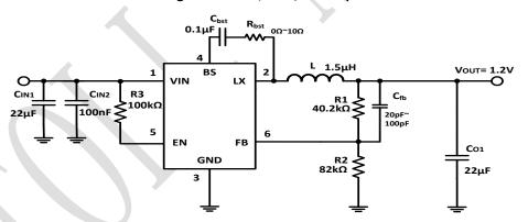
Figure 8. 12V<sub>IN</sub>, 1.2V/2A Output
