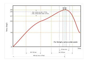
Fig 2. Infrared soldering profile
