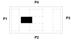
PINConnectionPINConnection1Input port3Output port2GND4GND
