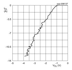
Pin C2;  $t_p = 100$  ns; Transmission Line Pulse (TLP)
