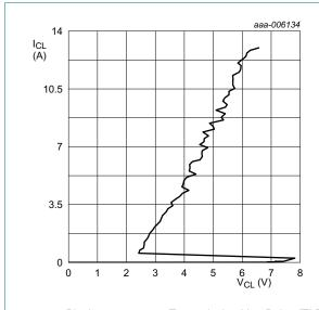
Pin A2; t<sub>p</sub> = 100 ns; Transmission Line Pulse (TLP)
