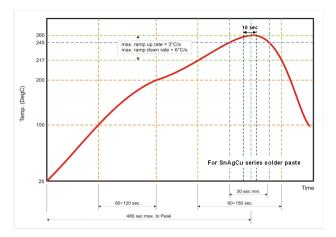
Fig 2. Infrared soldering profile
