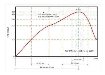
Fig 2. Infrared soldering profile
