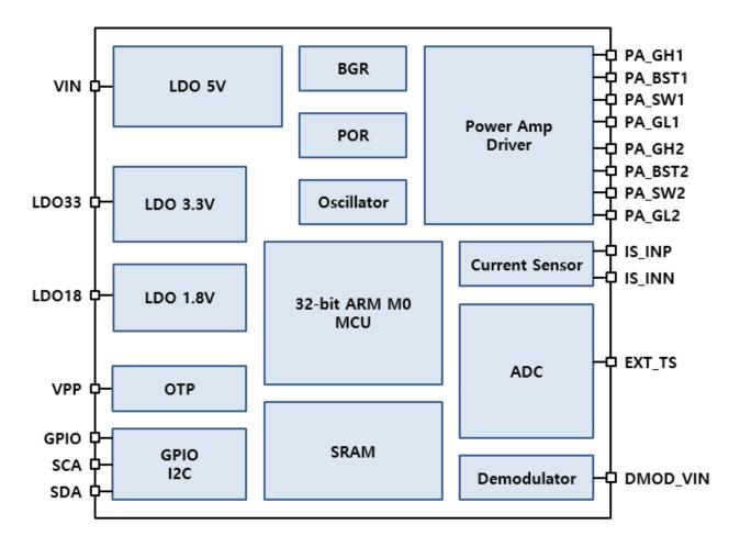
Figure 1. CWT1000 Block Diagram
