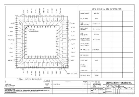
Figure 5. QFN 40-pin Bonding Diagram
