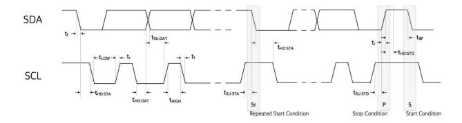
Figure 6. Timing Diagram for I<sup>2</sup>C interface
