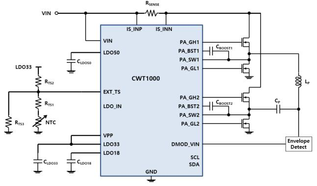
Figure 3. CWT1000 Typical Application Diagram
