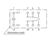
PC board mounting hole layout (BOTTOM VIEW)
