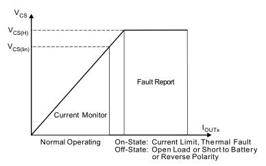
Figure 22. Current-Sense Output-Voltage Curve
