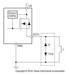
Figure 28. Protection With External Circuitry
