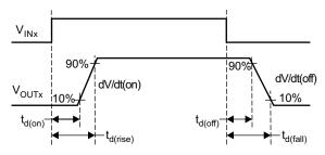
Figure 1. Output Delay Characteristics
