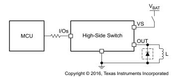
Figure 32. Protection for Loss of Power Supply, Method 2
