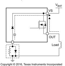
Figure 34. Reverse-Current External Protection, Method 2
