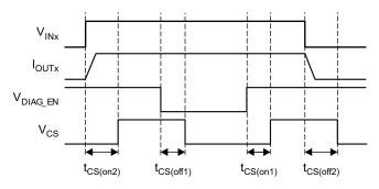
Figure 2. CS Delay Characteristics
