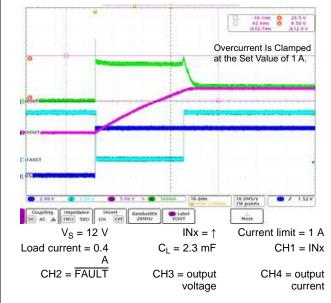
Figure 38. Driving a Capacitive Load With Adjustable Current Limit
