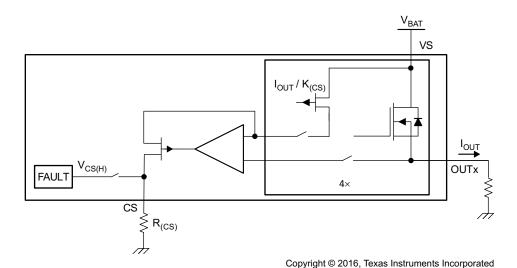
Figure 21. Current-Sense Block Diagram
