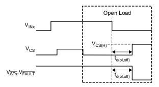
Figure 3. Open-Load Blanking-Time Characteristics
