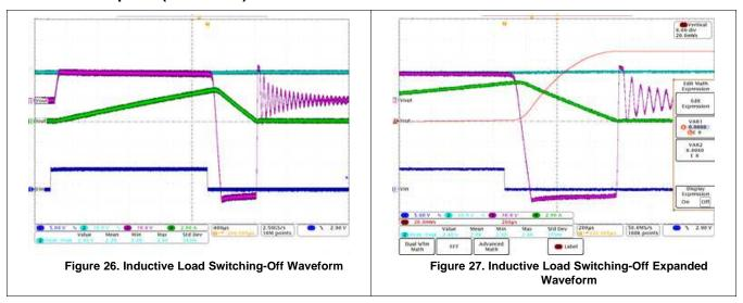
Note that for PWM-controlled inductive loads, it is recommended to add the external freewheeling circuitry shown in Figure 28 to protect the device from repetitive power stressing. TVS is used to achieve the fast decay. See Figure 28 for more details.
