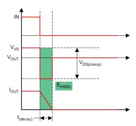
Figure 25. Inductive Load Switching-Off Diagram
