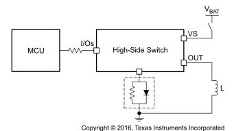
Figure 31. Protection for Loss of Power Supply, Method 1
