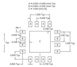
Note: Thermal vias for center slug "C" should be incoporated into the PCB design. The number and size of thermal vias will depend on the application. Example of the number and size of vias can be found on the RFMD evaluation board layout.
