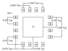
Note: Thermal vias for center slug "C" should be incoporated into the PCB design. The number and size of thermal vias will depend on the application. Example of the number and size of vias can be found on the RFMD evaluation board layout.
