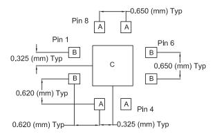
Note: Thermal vias for center slug "C" should be incorporated into the PCB design. The number and size of thermal vias will depend on the application. Example of the number and size of vias can be found on the RFMD evaluation board layout.
