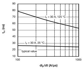
Fig. 7 - Typical Reverse Recovery vs. dl<sub>E</sub>/dt
