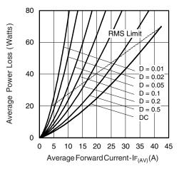
Fig. 6 - Forward Power Loss Characteristics
