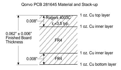
50 ohm line dimensions: width = 0.0182", spacing = 0.020"
