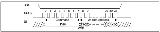
Figure 50.64KB Block Erase Sequence Diagram (ADS=1)
