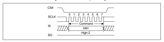
Figure 6. Write Disable Sequence Diagram
