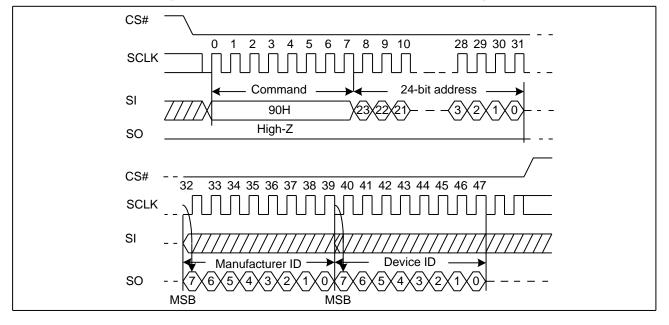
Figure 61. Read Manufacture ID/ Device ID Sequence Diagram
