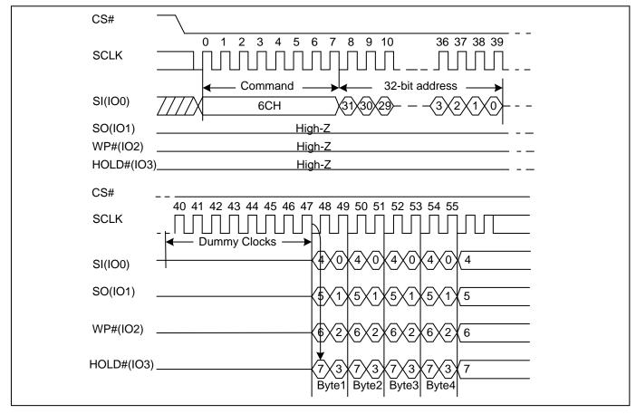
1. The dummy clock number is configurable.
