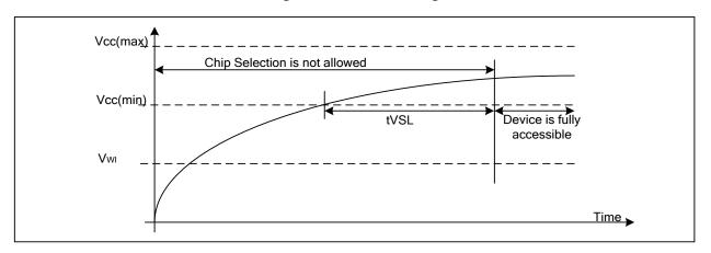
Table 25. Power-Up Timing and Write Inhibit Threshold
