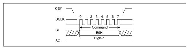
Figure 57.Exit 4-Byte Address Mode Sequence Diagram
