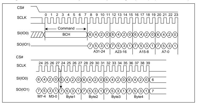
1. The dummy clock number is configurable.
