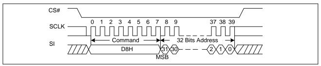
Figure 51. 64KB Block Erase with 4-Byte Address Sequence Diagram (ADS=0 or ADS=1)
