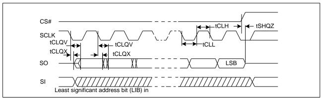
Figure 80. Resume to Suspend Timing
