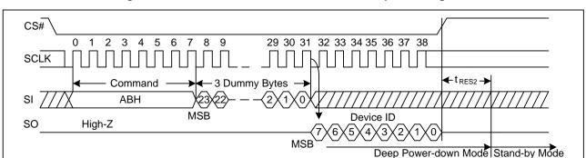
Figure 60. Release Power-Down/Read Device ID Sequence Diagram
