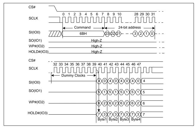
Figure 21. Quad Output Fast Read Sequence Diagram (ADS=0)
