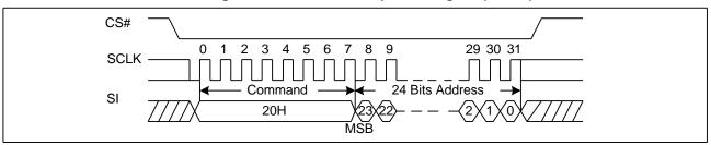
Figure 44. Sector Erase Sequence Diagram (ADS=1)
