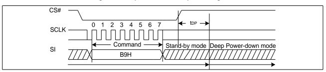
Figure 53. Deep Power-Down Sequence Diagram
