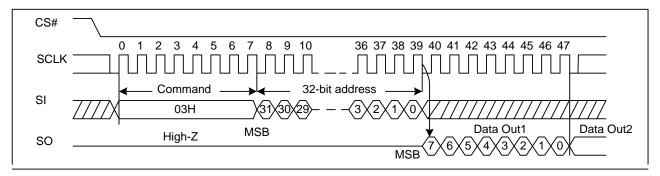
Figure 14. Read Data with 4-Byte Address Sequence Diagram (ADS=0 or ADS=1)
