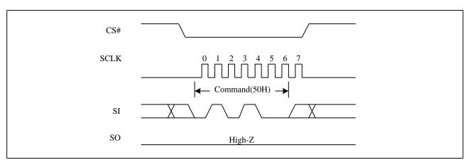
Figure 7. Write Enable for Volatile Status Register Sequence Diagram
