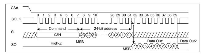
Figure 13. Read Data Bytes Sequence Diagram (ADS=1)
