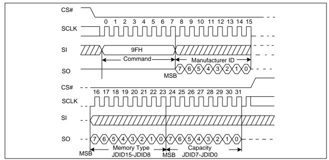
Figure 64. Read Identification ID Sequence Diagram
