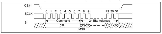
Figure 47.32KB Block Erase Sequence Diagram (ADS=1)
