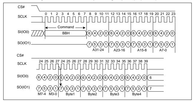
1. The dummy clock number is configurable.
