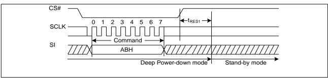
Figure 59. Release Power-Down Sequence Diagram
