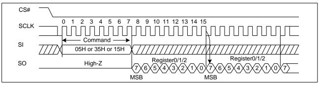
Figure 8. Read Status Register Sequence Diagram
