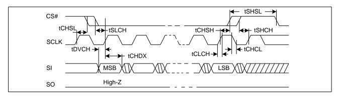
Figure 79. Output Timing
