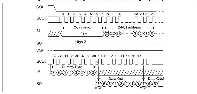
Figure 72. Read Security Registers command Sequence Diagram (ADS=1)
