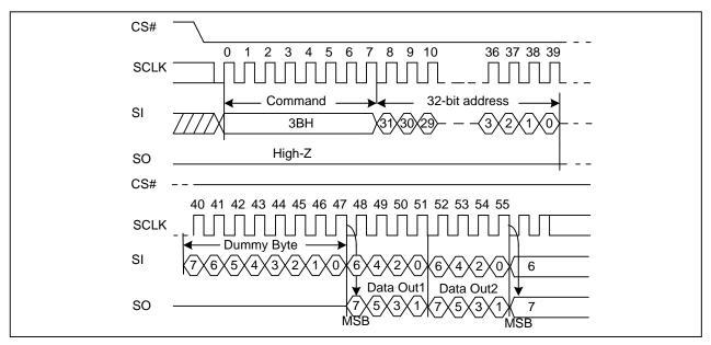
1. The dummy clock number is configurable.
