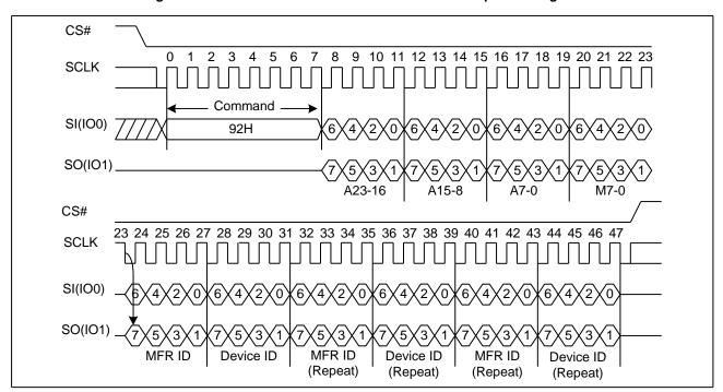
Figure 62. Read Manufacture ID/ Device ID Dual I/O Sequence Diagram
