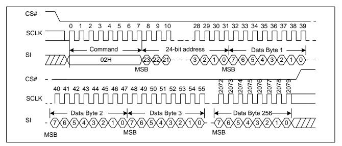
Figure 37. Page Program Sequence Diagram (ADS=0)
