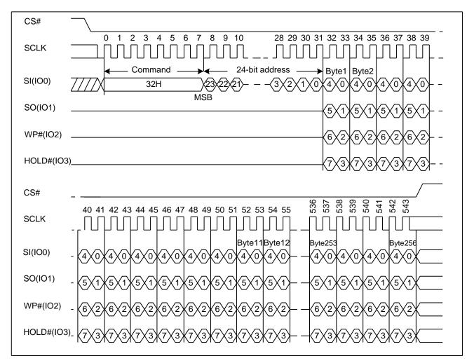
Figure 40. Quad Page Program Sequence Diagram (ADS=0)
