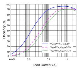
Figure 2. Efficiency vs. Load Current
