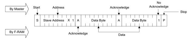
Figure 13. Hs-mode Current Address Read
