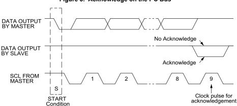
Figure 5. Acknowledge on the I<sup>2</sup>C Bus
