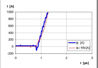
Fast increasing currents (higher than the specified  $I_{p,max}$ ), e.g. in case of a short circuit, can be transmitted because the currents are transformed directly.
