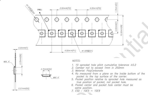
Figure 8 Tape and reel dimensions
