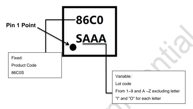
Figure 7 Marking specification (Top View)
