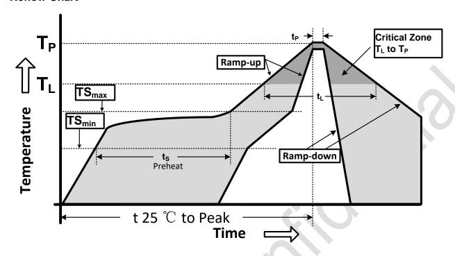
Figure 9 Recommended Lead-Free Reflow Profile
