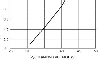
Figure 2. Clamping Voltage vs Peak Pulse Current
