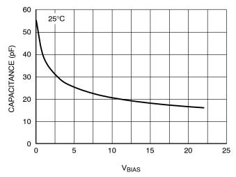
Figure 5. Capacitance vs.  $V_{BIAS}$
