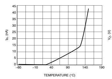
Figure 3. Typical Leakage vs. Temperature
