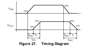
w here:  $td_{ON} = Delay$  On Time  $t_R = V_{OUT}$  Rise Time  $t_{ON} = Turn-On$  Time  $td_{OFF} = Delay$  Off Time  $t_F = V_{OUT}$  Fall Time  $t_{OFF} = Turn-Off$  Time
