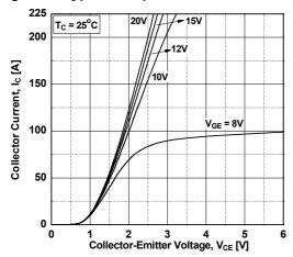
Figure 3. Typical Saturation Voltage Characteristics
