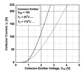
Figure 5. Saturation Voltage vs. V<sub>GE</sub>
