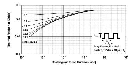
Figure 22. Transient Thermal Impedance of Diode
