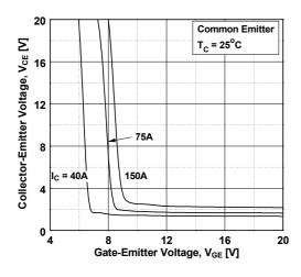
**Figure 2. Typical Output Characteristics**
