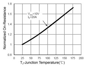
Figure 4 Rdson-JunctionTemperature
