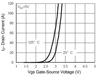
**Figure 2 Transfer Characteristics**
