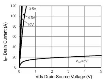
**Figure 1 Output Characteristics**
