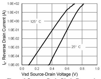
Figure 6 Source- Drain Diode Forward
