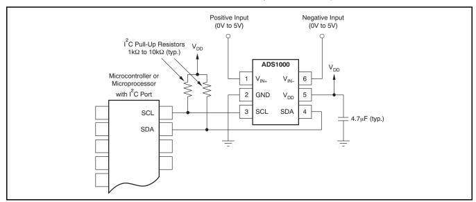
Figure 9. Typical Connections of the ADS1000
