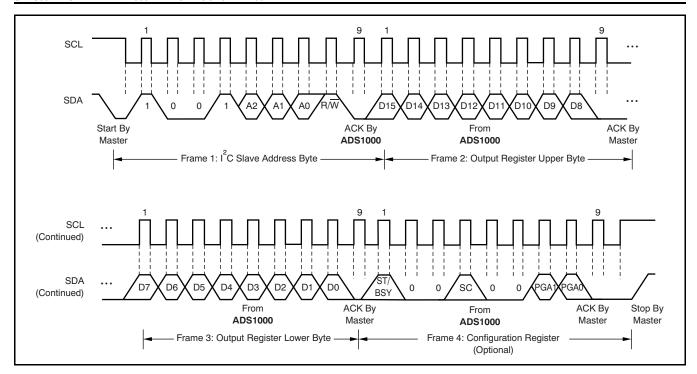
Figure 7. Timing Diagram for Reading from the ADS1000
