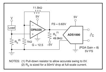
Figure 13. Low-Side Current Measurement
