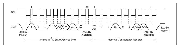
Figure 8. Timing Diagram for Writing to the ADS1000
