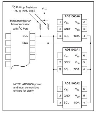
Figure 10. Connecting Multiple ADS1000s
