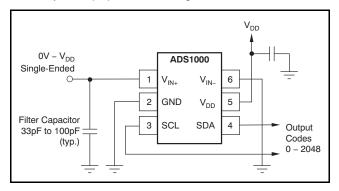
Figure 12. Measuring Single-Ended Inputs
