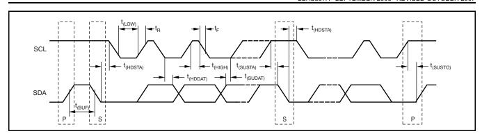
Figure 6. I<sup>2</sup>C Timing Diagram
