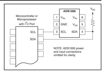
Figure 11. Using GPIO with a Single ADS1000
