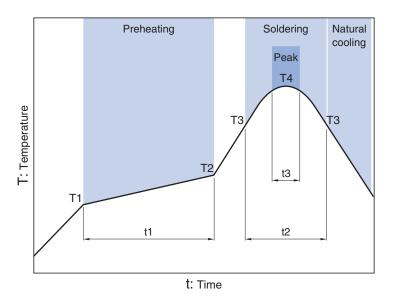
Preheating Soldering Peak Temp. Temp. Temp. Time Time Time **T1** T2 Т4 t1 ТЗ t2 t3 150°C 180°C 60 to 120s 230°C 30 to 60s 250 to 260°C 10s max.
