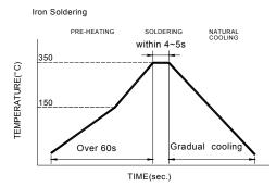
Iron Soldering times: 1 times max.
