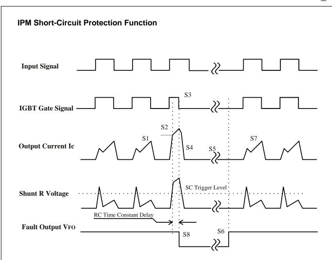
Figure 11. Timing Chart of SC Operation
