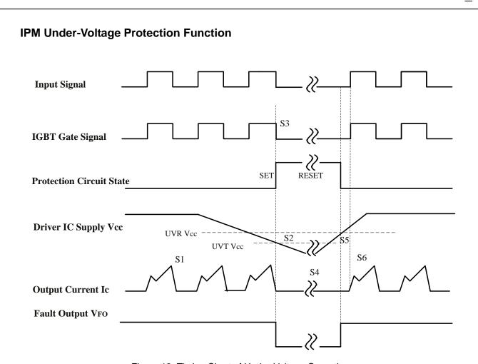
Figure 12. Timing Chart of Under-Voltage Operation
