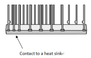
Figure 8. Measurement Location of Heat-sink Flatness
