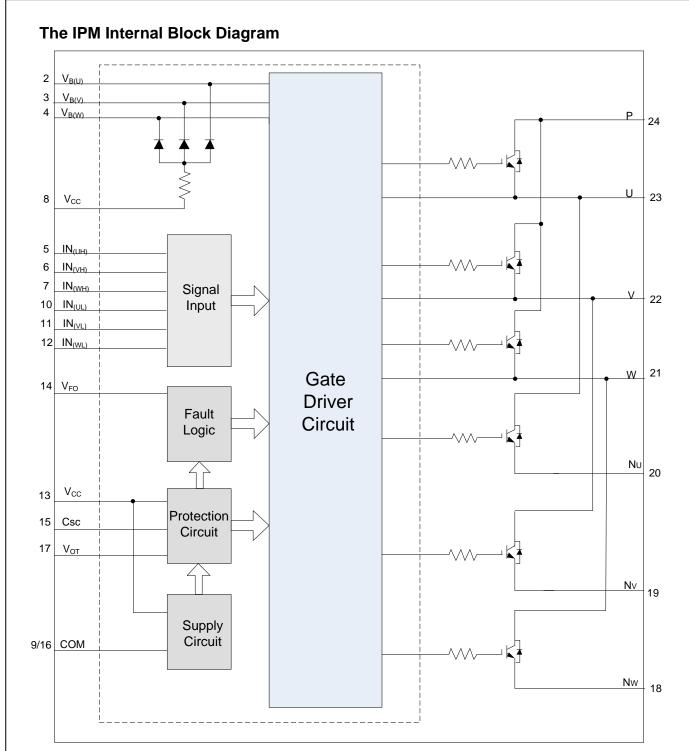
Figure 3. IPM Internal Block Diagram
