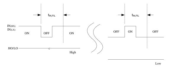
Figure 6. Input Filter Function
