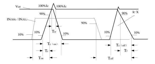
Figure 5. Switching Time Definition
