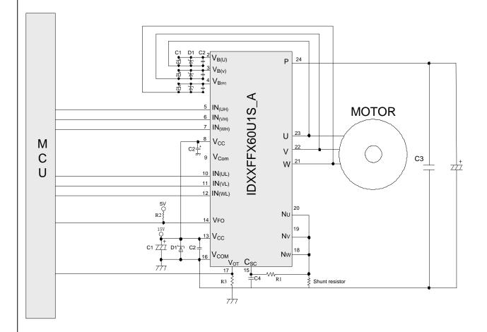
Figure 13. Typical Application Circuit Interface Example without Photo-Coupler
