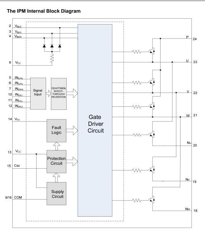
Figure 3. IPM Internal Block Diagram
