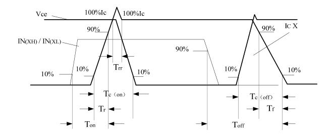
Figure 5. Switching Time Definition
