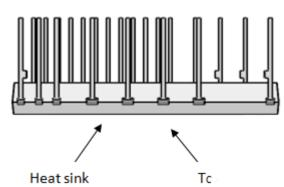
Figure 4. Tc Measurement Point
