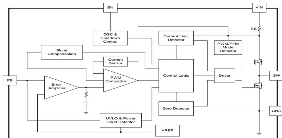
Figure 1. H9008 Block Diagram
