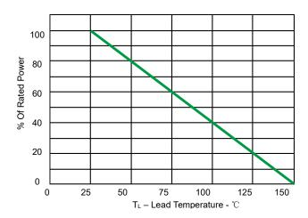
Fig 2.Power Derating Curve
