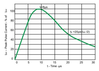
Fig 1.Pulse Waveform
