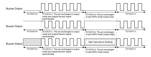
Example: Setup TC1OUT output from TC1 to TC1OUT (P5.3). The external high-speed clock Fhosc is 4MHz. the instruction cycle Fcpu is Fhosc/4. The TC1OUT frequency is 0.5KHz. Because the TC1OUT signal is divided by 2, set the TC1 clock to 1KHz. The TC1 clock source is from external oscillator clock. TC1 rate is Fcpu/8. The TC1RATE2~TC1RATE1 = 101. TC1C = TC1R = 131.
