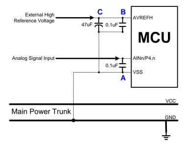
The analog signal is inputted to ADC input pin "AINn/P4.n". The ADC input signal must be through a 0.1uF capacitor "A". The 0.1uF capacitor is set between ADC input pin and VSS pin, and must be on the side of the ADC input pin as possible. Don't connect the capacitor's ground pin to ground plain directly, and must be through VSS pin. The capacitor can reduce the power noise effective coupled with the analog signal.
