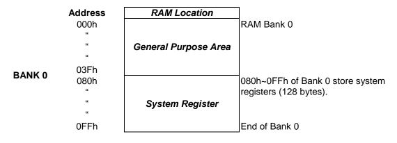
The 64-byte general purpose RAM is in Bank 0. Sonix provides "Bank 0" type instructions (e.g. b0mov, b0add, b0bts1, b0bset...) to control Bank 0 RAM in non-zero RAM bank condition directly.
