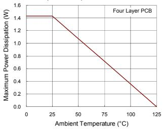
Figure 2. Derating Curve of Maximum Power Dissipation
