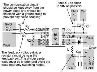
Place the power components as close to the IC as possible. The traces should be wide and short, especially for the high-current loop.
