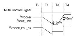
Figure 13. VDDCR\_FCH\_S5 Simplified Timing Diagram
