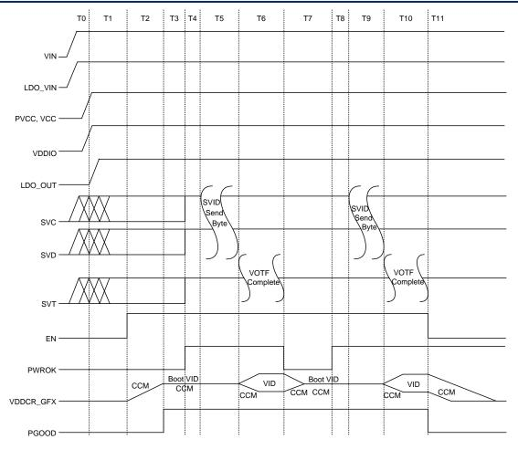
Figure 2. Simplified Sequence Timing Diagram
