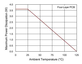
Figure 15. Derating Curve of Maximum Power Dissipation
