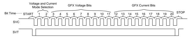
Figure 3. Telemetry Bit Definition
