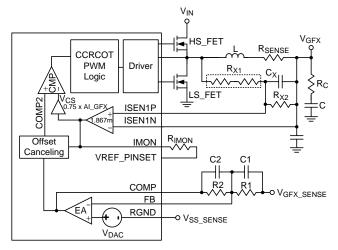
Figure 7.GFX Controller : Simplified Schematic with Voltage Loop and Current Loop
