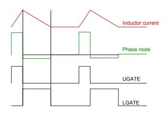
Figure 2. Diode Emulation Mode (DEM) in Steady State
