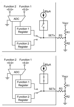
Figure 5. Multi-Function Pin Setting Mechanism with a R3 Resistor to Fine Tune the Set Voltage of Function2
