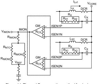
Figure 14. Thermal Compensation method for dual Phase
