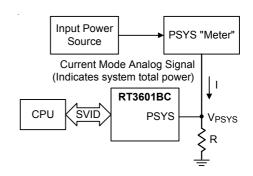
Figure 20. PSYS Function Block Diagram
