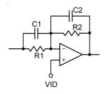
Figure 18. Type I compensator
