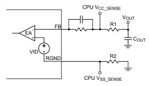
Figure 19. Remote Sensing Circuit
