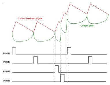
Figure 1 (b). G-NAVP<sup>™</sup> Behavior Waveforms in CCM in Load Transient.
