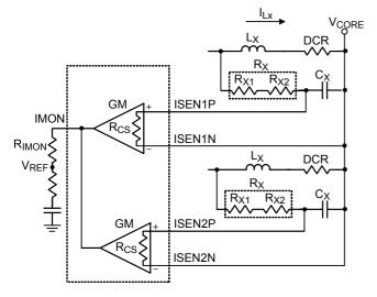
Figure 12. Lossless Current Sense Method for Dual Phase
