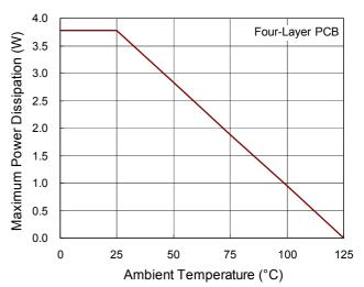
Figure 27. Derating Curve of Maximum Power Dissipation
