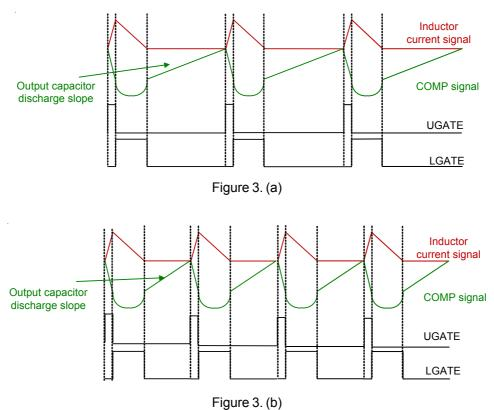
Figure 3. G-NAVP<sup>TM</sup> Operation in DEM. (a) : The load is lighter, output capacitor discharge slope is smaller and the switching frequency is lower. (b) : The load is increasing, output capacitor discharge slope is increased and switching
