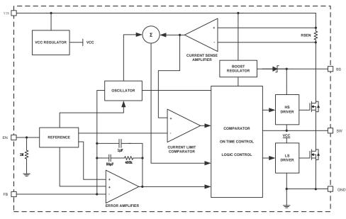
Figure 2. RY3834 Block Diagram
