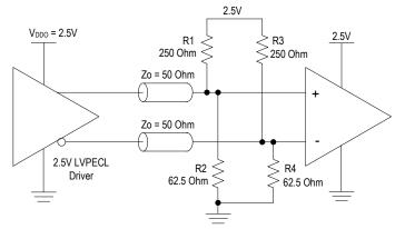
Figure 16. 3.3V LVPECL Output Termination (2)
