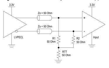
Figure 17. 2.5V LVPECL Output Termination
