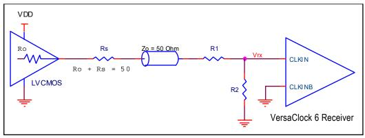
Table 25 shows resistor values that ensure the maximum drive level for the CLKIN port is not exceeded for all combinations of 5% tolerance on the driver  $V_{DD}$ ,  $V_{DDO0}$  and 5% resistor tolerances. The values of the resistors can be adjusted to reduce the loading for slower and weaker LVCMOS driver by increasing the impedance of the R1–R2 divider. To better assist this assessment, the total load (Ro + Rs + R1 + R2) on the driver is included in the table.
