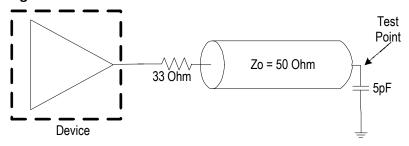
Figure 3. HCSL Test Load
