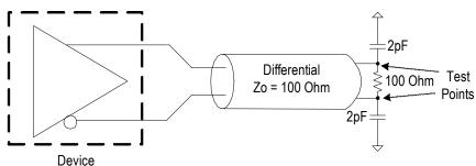
Figure 5. LVPECL Test Load
