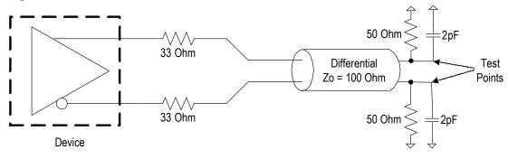
Figure 4. LVDS Test Load
