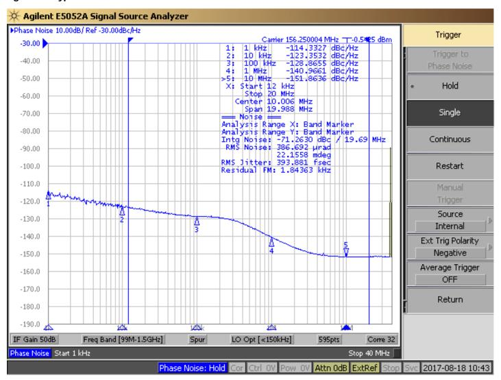
Note: Measured with OUT2 = 156.25MHz on, 39.625MHz input.
