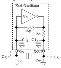
Cs1 and Cs2 are stray capacitances at each crystal pin and typical values are between 1pF and 3pF.
