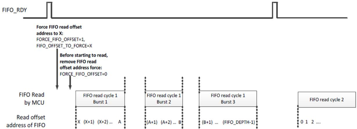
Figure 20. Recommended Method to Deassert FORCE\_FIFO\_OFFSET When Using Multiple Read Bursts to Read the FIFO
