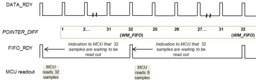
Figure 25. FIFO mode based on programmable watermark level
