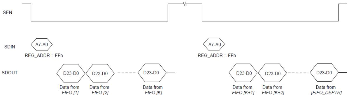
Figure 42. FIFO readout over two read operation
