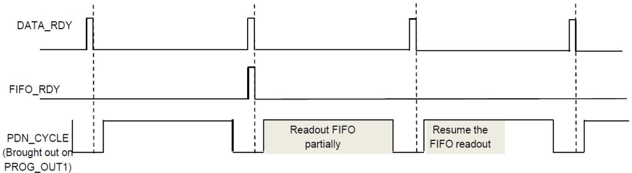
Figure 24. FIFO readout over multiple PDN\_CYCLE phases
