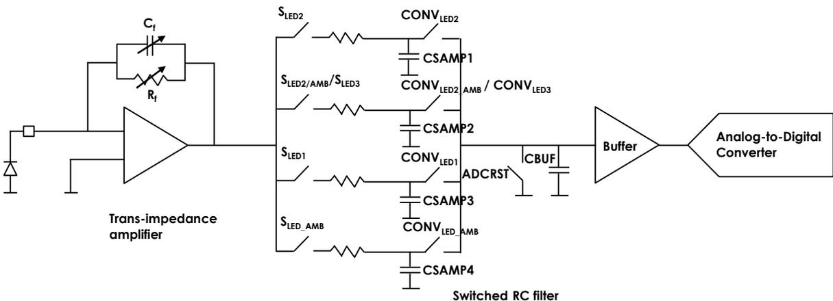
Figure 8. Illustration of the noise reduction filter
