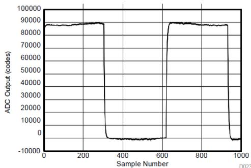
Figure 48. Ambient data with ambient light modulation
