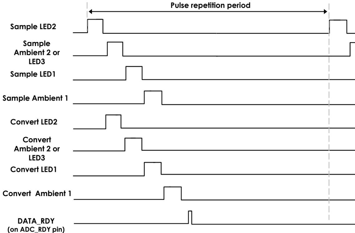
Figure 3. Sequence of Four Sampling and Conversion Phases
