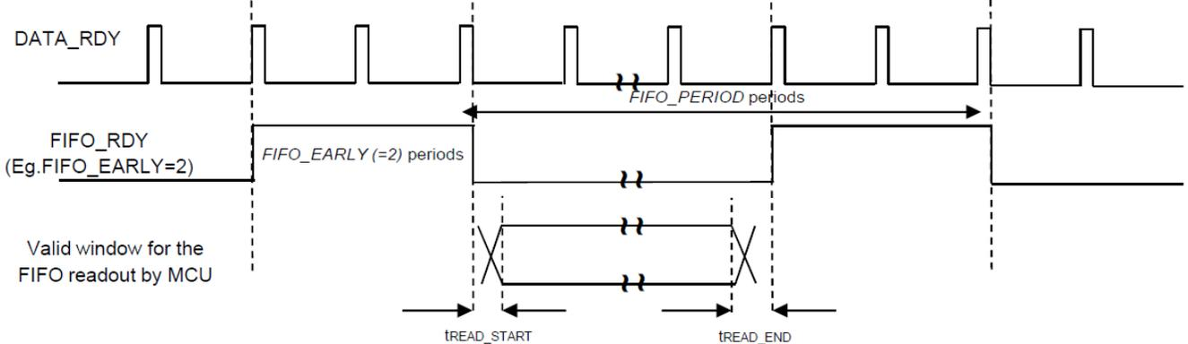
Figure 22. Time window for the MCU to read the FIFO
