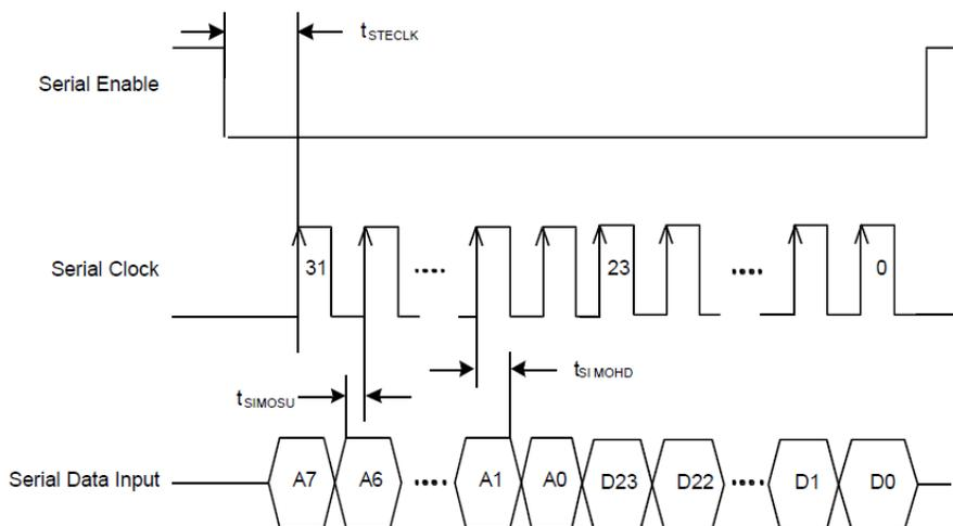
Figure 2. Serial Interface Timing Diagram, Write Operation
