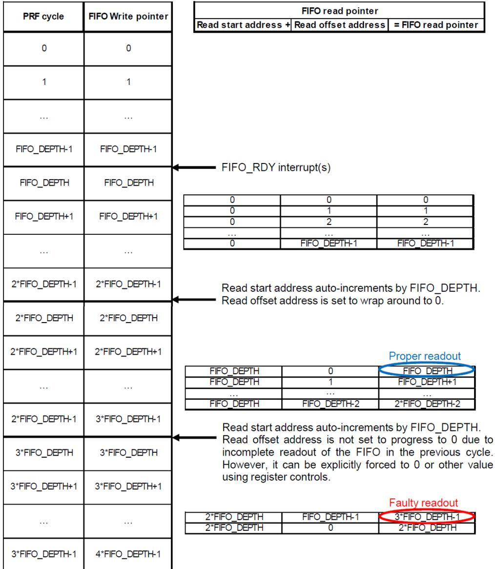
Figure 17. Progression of FIFO read and write pointer
