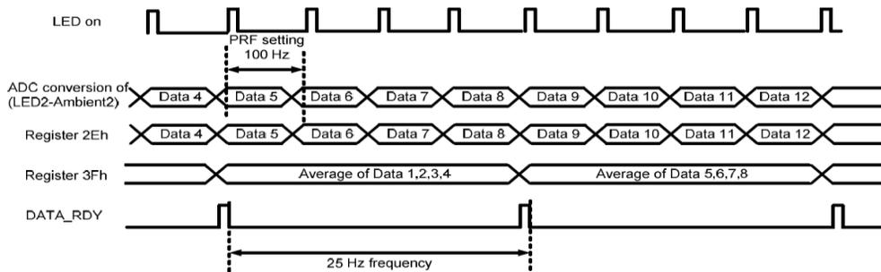
Figure 27. Decimation mode Timing diagram (Decimation factor=4, PRF=100Hz)
