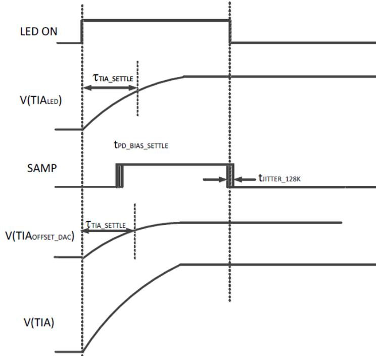
Figure 52. TIA settling transient with EARLY\_OFFSET\_DAC set to '1'
