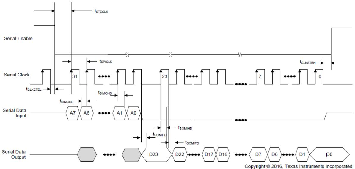
Figure 1. Serial Interface Timing Diagram, Read Operation
