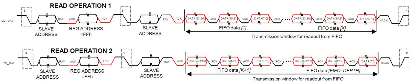
Figure 36. I<sup>2</sup>C Readout from FIFO over two read operations
