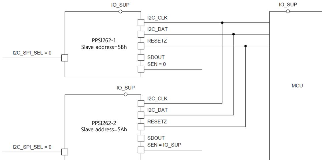
Figure 54. Connection of two PPSI262s to the MCU when operating in I<sup>2</sup>C mode
