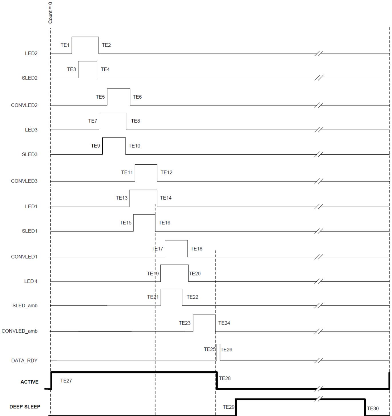
Figure 13. Timing Diagram of various programmable signal phases
