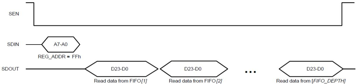
Figure 41. Continuous FIFO readout through the SPI interface
