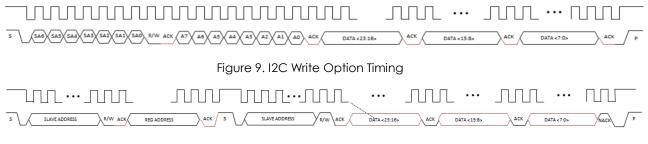
Figure 10. I2C Read Option Timing
