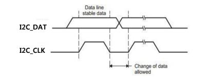
Figure 7. Allowed Window for Data Transition
