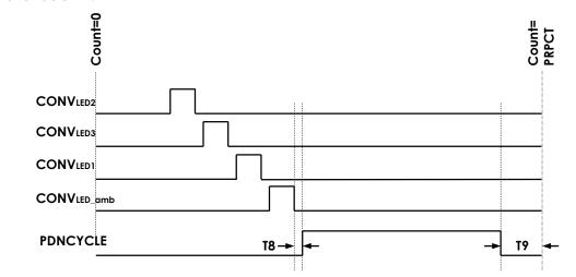
The dynamic powerdown feature can be used to shut down the receiver inside every cycle to save power. See Figure 14 and Table 11.
