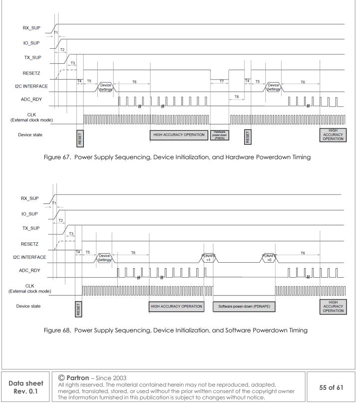
The guidelines for Power supply sequencing and Device initialization are shown in Figure 67 and Figure 68.
