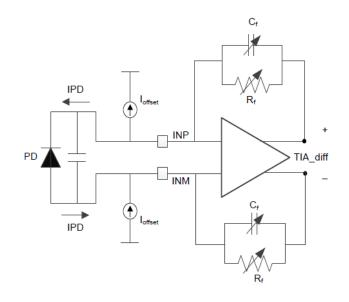
With the photodiode connected as shown, In figure 5, the output code of the PPS964A would be positive with the offset cancellation DAC set to zero (loffset=0). With loffset set negative (POL\_OFFFAC=1), a DC offset can be subtracted from the signal, and the AC signal could be amplified with a higher gain than would be otherwise possible.
