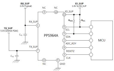
Figure 68. Hardware pin connection diagram in external clock mode
