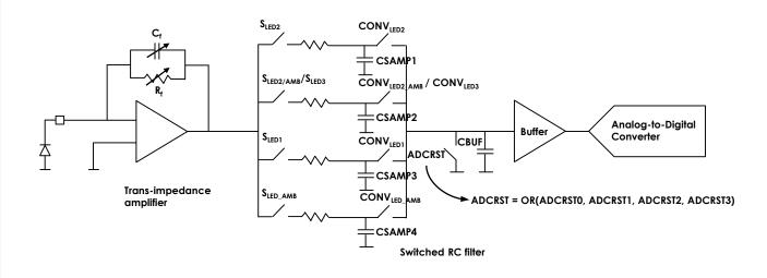
Figure 3. Illustration on Four Phases of Sampling and Conversion
