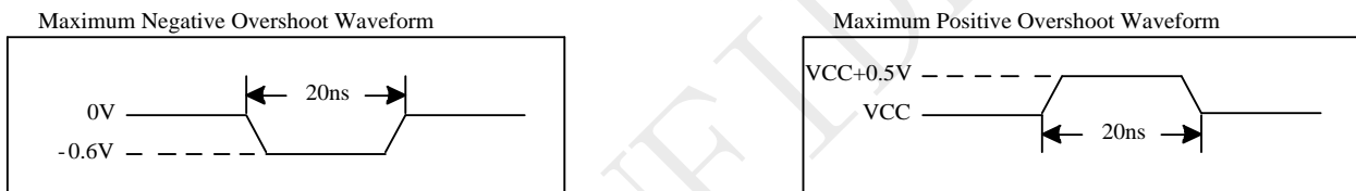
Figure 5-1 Maximum Overshoot Waveform
