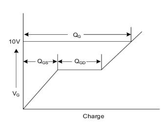
Fig. 3.2 Gate Charge Waveform
