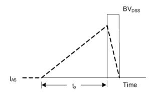
Fig. 4.2 Unclamped Inductive Switching Waveforms
