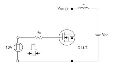
Fig. 4.1 Unclamped Inductive Switching Test Circuit
