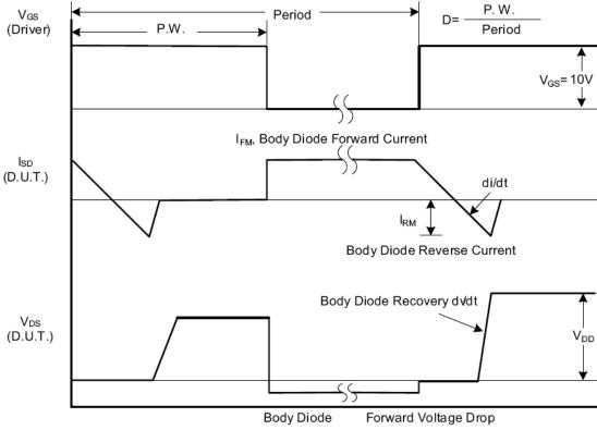
Fig. 1.2 Peak Diode Recovery dv/dt Waveforms
