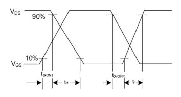
Fig. 2.2 Switching Waveforms
