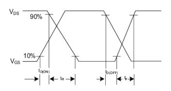
Fig. 2.2 Switching Waveforms
