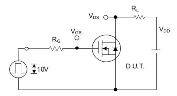
Fig. 2.1 Switching Test Circuit
