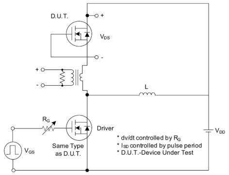
Fig. 1.1 Peak Diode Recovery dv/dt Test Circuit
