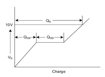
Fig. 3.2 Gate Charge Waveform
