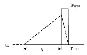
Fig. 4.2 Unclamped Inductive Switching Waveforms
