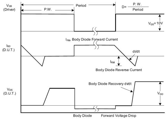
Fig. 1.2 Peak Diode Recovery dv/dt Waveforms
