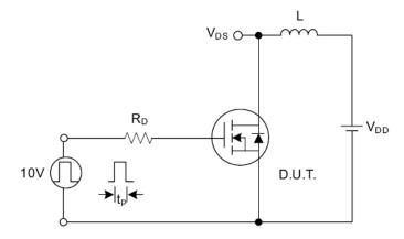
Fig. 4.1 Unclamped Inductive Switching Test Circuit
