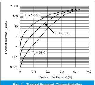
Fig. 1. Typical Forward Characteristics
