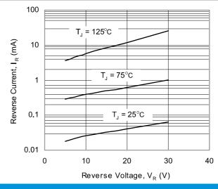
Fig. 2. Typical Reverse Characteristics
