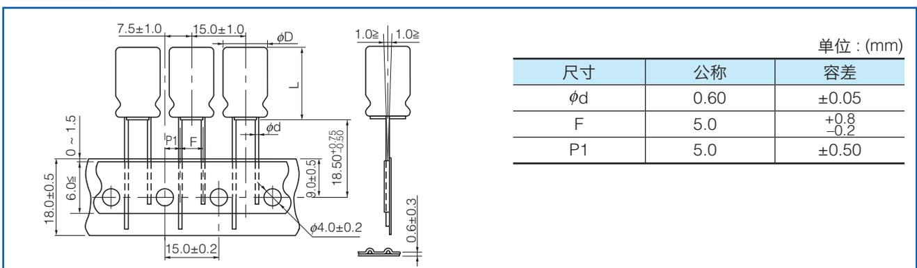
**类别 H** (引线间距: 7.5 mm /  $\phi D \times L$ :  $\phi 16 \times 15, 20, 25, \phi 18 \times 15, 20, 25$ )
