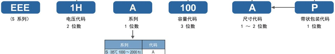
Note) \* If part number exceeds 12 figures, voltage code is abbreviated as follows, 0J → J, 1A → A, 1C → C, 1E → E, 1V → V, 1H → H
