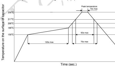
Note: \*Measurement position of temperature: The top of capacitor and terminal
