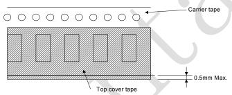
(2) In case the top cover tape covers a part of sprocket hole, the distance shall not exceed 0.75mm.
