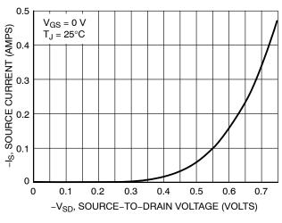
Figure 10. Diode Forward Voltage vs. Current
