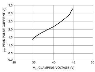
Figure 2. Clamping Voltage vs Peak Pulse Current
