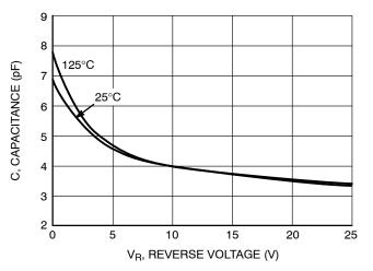
Figure 3. Typical Junction Capacitance vs
