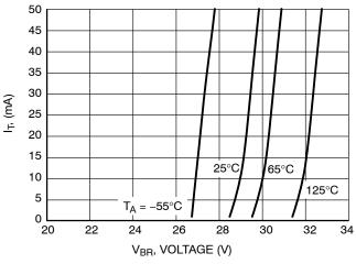
Figure 4. V<sub>BR</sub> versus I<sub>T</sub> Characteristics
