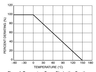
Figure 6. Temperature Power Dissipation Derating
