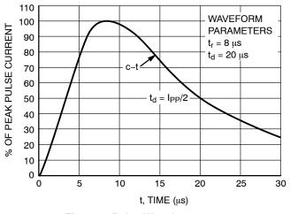
Figure 1. Pulse Waveform, 8  $\times$  20  $\mu s$
