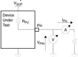
Figure 6. Internal Resistor Test Conditions,  $T_A = 0$ °C to 70°C
