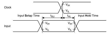
Figure 9. Input Setup and Hold Time
