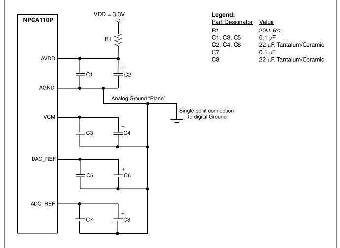
Figure 4. Recommended CODEC Power Connection Diagram
