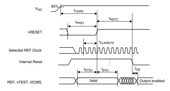
Figure 11. Device Reset
