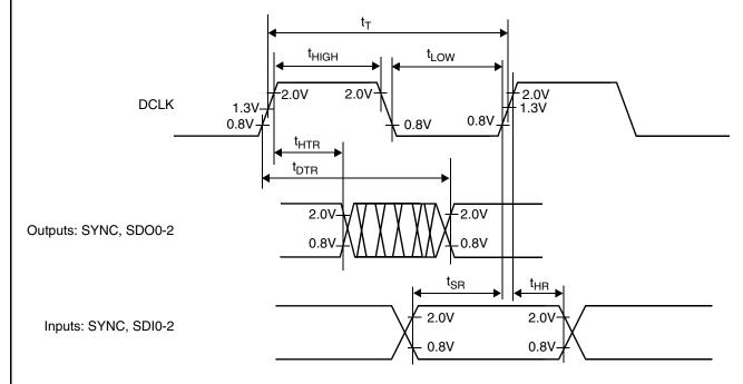
Figure 17. SSI Signal Timing
