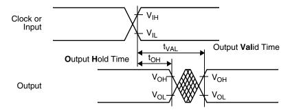
Figure 10. Clock-to-Output and Propagation Delay
