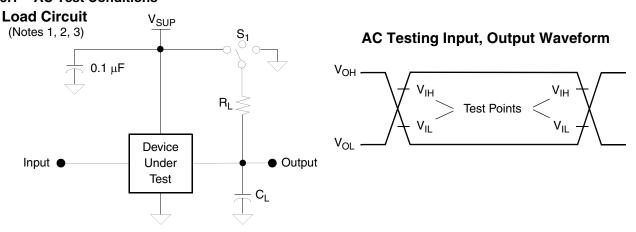
Figure 8. AC Test Conditions,  $T_A = 0^{\circ}C$  to  $70^{\circ}C$ ,  $V_{SUP} = 3.13V - 3.47V$
