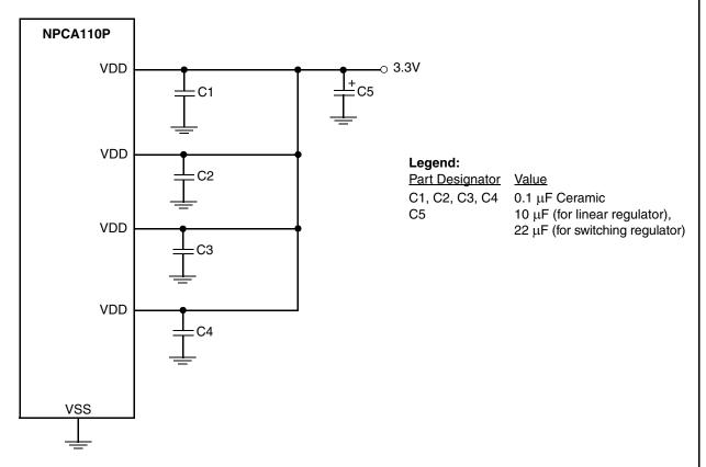
Figure 1. 3.3V Digital Power Connection Diagram
