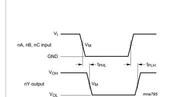
$V_M$  = 1.5 V at  $V_{CC} \ge 2.7$  V.
