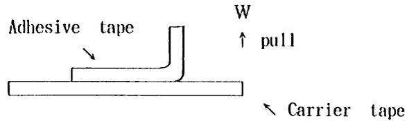
3-6. Tensile test : When pulling a test sample by the force 10N, there shall be no gaps or breakdowns.
