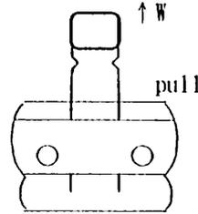
3-7. Moisture resistance test : A taped test sample shall be left in a chamber with a temperature of 40°C and RH95% for 96 hours. Then after being left for one hour at room temperature, the test sample shall be submitted to a tensile test of item 3.6.
