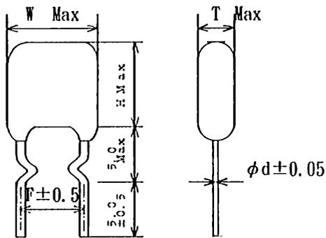
• MMT D : Double-formed lead type
